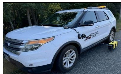
Mobile Pavement Marking Retroreflectometer and Camera System
