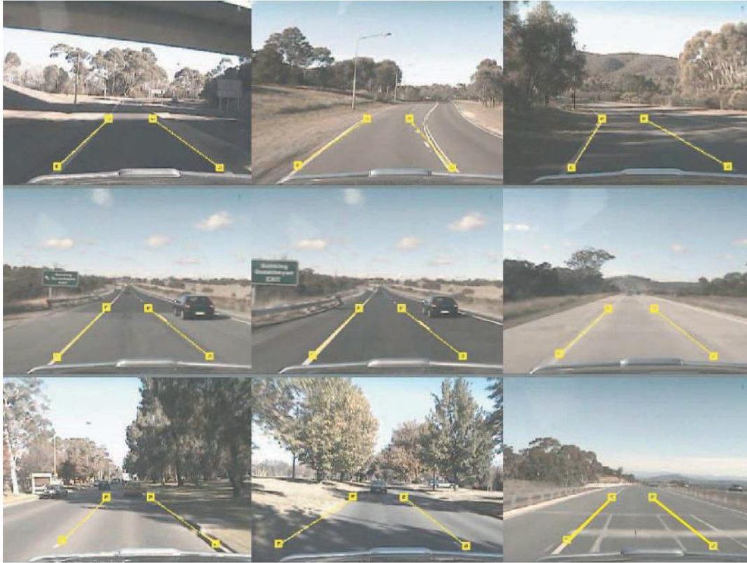
Figure 8. Lane tracking algorithm showing the estimated lane boundary against shadows, obstacles, and misleading markings (82)
