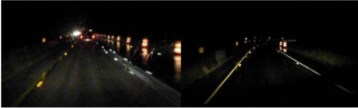
Figure 6. Wet weather comparison of standard pavement marking (left) and the AWP (right) pavement markings (22)
