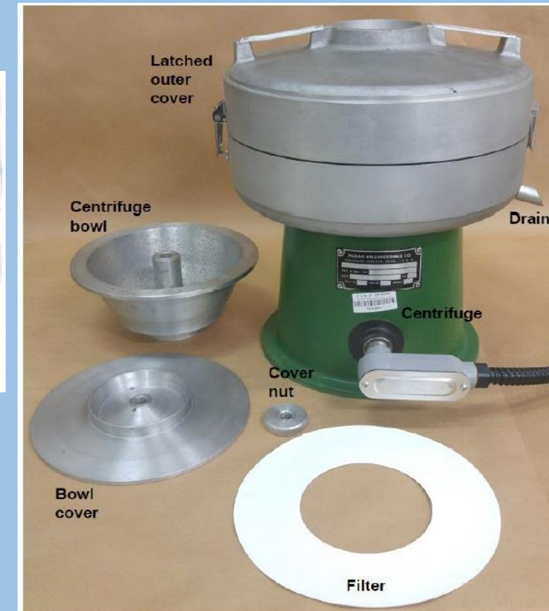
Figure 1—Centrifuge Apparatus (Source: LTRC/DOTD)
