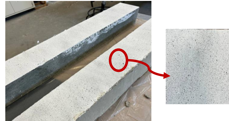
Surface preparation of concrete beams for DIC
